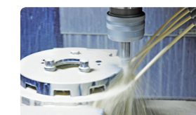
Bell housing machining by the MCT
