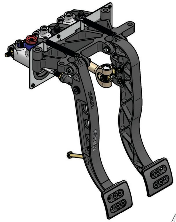
LONG CLEVIS FOR LONGER STROKE FRONT MASTER CYLINDER AT REST, LONG CLEVIS ROTATES BIAS BAR AS SHOWN. THIS ALLOWS BIAS BAR TO RUN SQUARE UNDER BRAKING.
